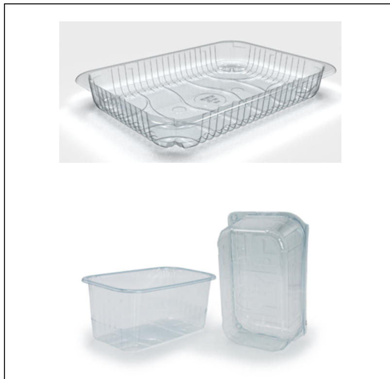
Figure 1: trays produced by thermoforming A/B/A sheets containing rPET in the B layer
