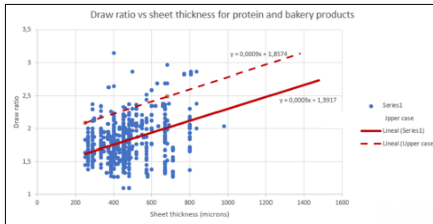
Figure 2(a). Most common distribution of draw ratios applied to produce thermoforms for protein and bakery products
