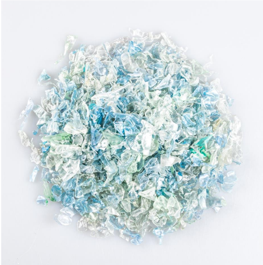
Purified Flakes from PCR PET Trays
