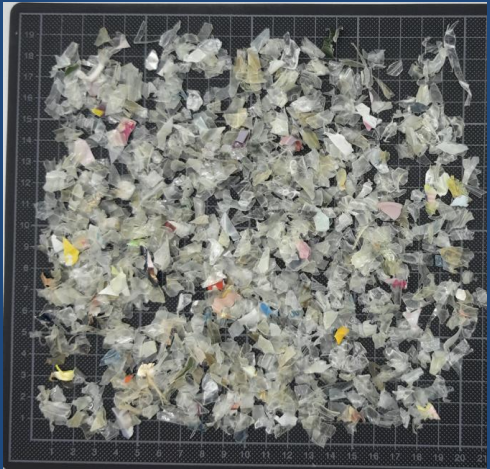
Example: Output PCR PET-Trays (without flake sorting)
