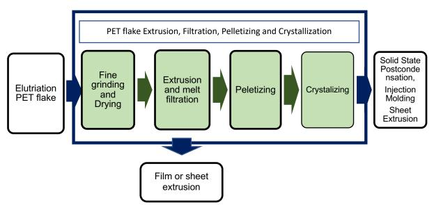
Note: Melt filtration and pressure measurement is not necessary when the practice is used only to add a heat history.
