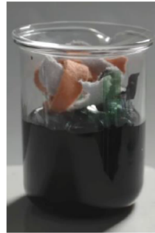
Step 2: Addition of Magnetic Fluid to PET materials and heating
