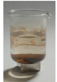
Step 3: Magnetic separation of the Magnetic Fluid: addition of water, magnetic sedimentation and decanting of supernatant
